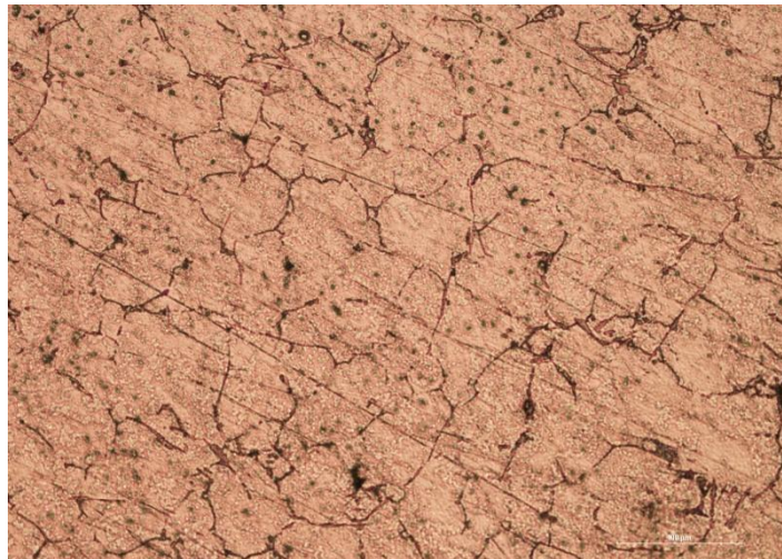
Fig. 2 - Microstructure (x200)of SiC reinforced Al.
