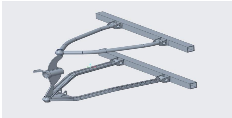
Figure 6: Complete Double Arm Suspension Model
