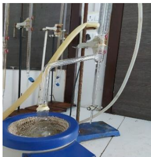
Figure. 1 - Dean and Stark Method for determination of water content
