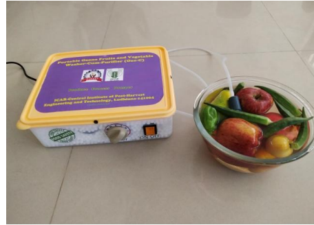
Fig. 2- Portable ozone fruits and vegetable washer-cum-purifier
