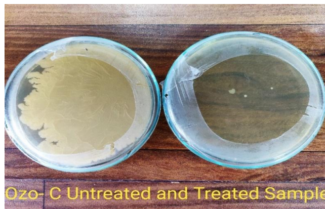
Fig. 4- Effect of ozonation on microbial population in tap water treated with ozone fruits and vegetable washer-cum-purifier
