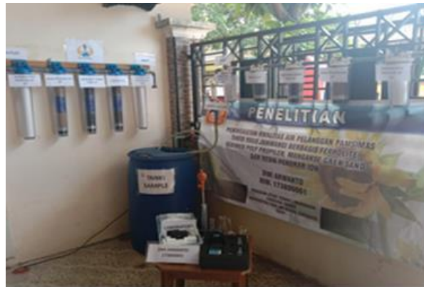
Fig. 2 – Installation of Micro Filtration
