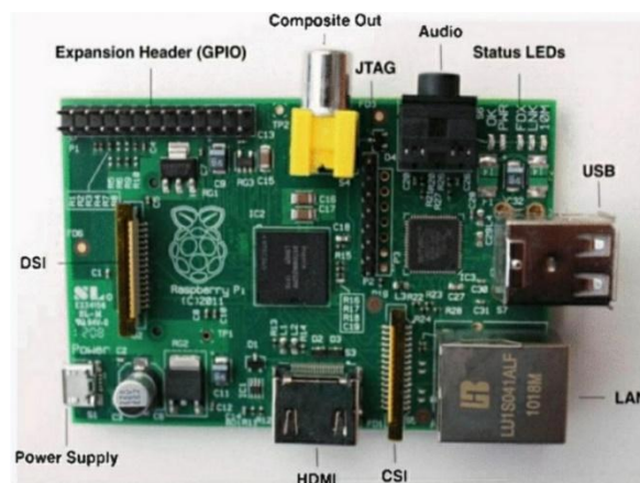
Fig. 3: Raspberry Pi board (Model-B).
