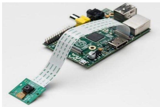
Fig. 4: Raspberry Pi camera board.
