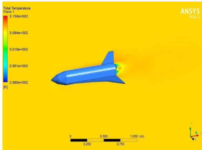
Fig.14 - Total Temperature Contour for ZrB 2 at Mach 1.5
