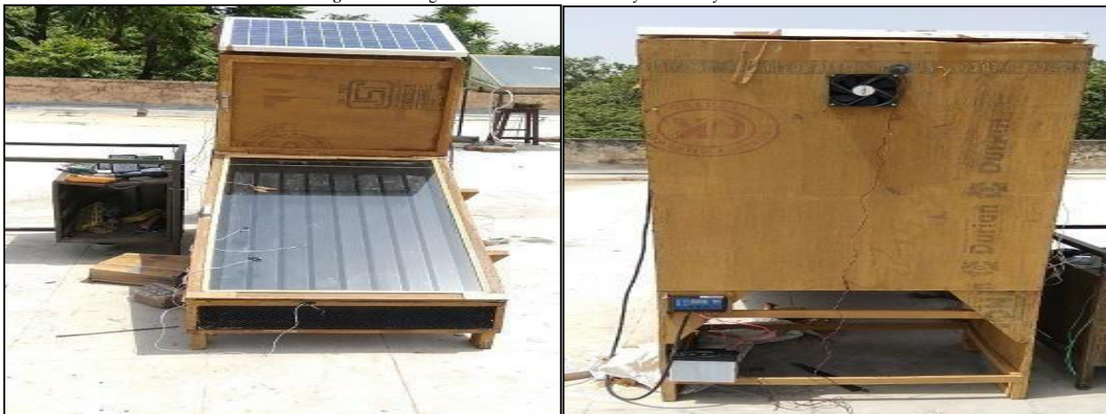
Fig. 4-Block diagram of solar air heater and dryer assembly
