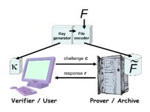
Figure 8. POR - Data Verification Process [40]
