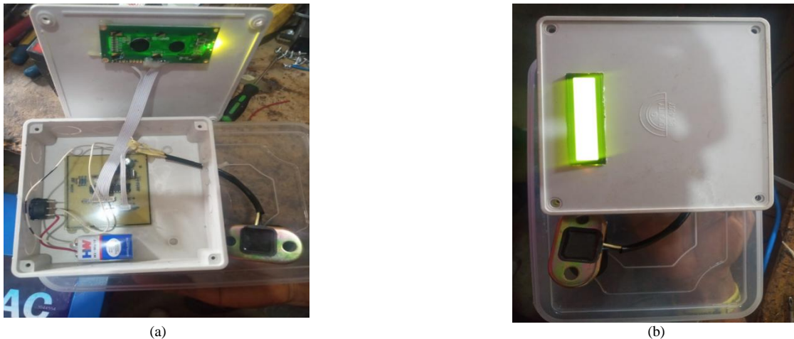
Figure 10: The proposed digital fuel level indicator (a) Internal connection (b) external features
