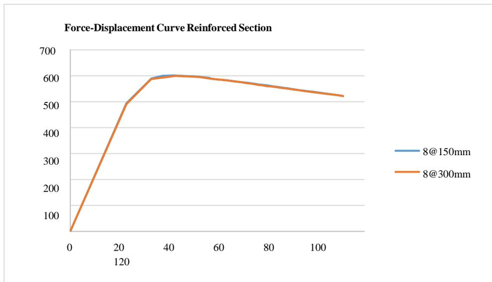
Figure 4.2 Force-Displacement Curve for Reinforced Section
