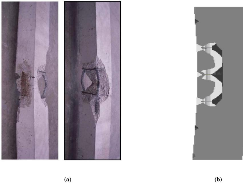
**Figure 3.5 Compression Damage in Column with Slenderness Ratio 40**
