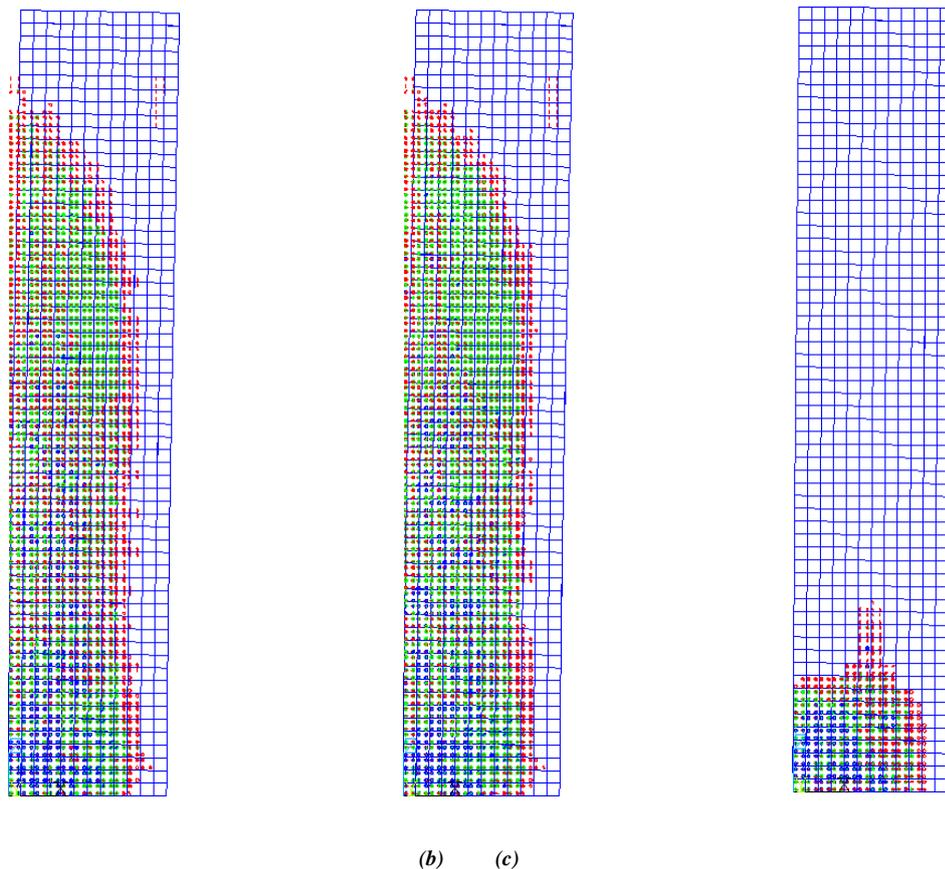
Figure 4.9 Crack Profile at Peak Loads (a) 150 mm Spacing (b) 300 mm Spacing (c) Unreinforced Concrete
