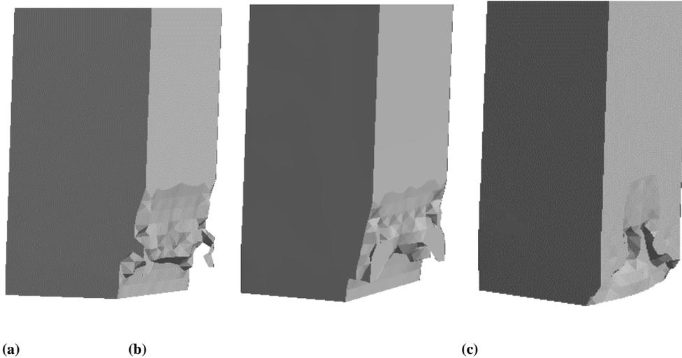
Figure 4.8 Concrete State at 100 mm Displacement for (a) 150 mm Spacing (b) 300 mm Spacing (c) Unreinforced
