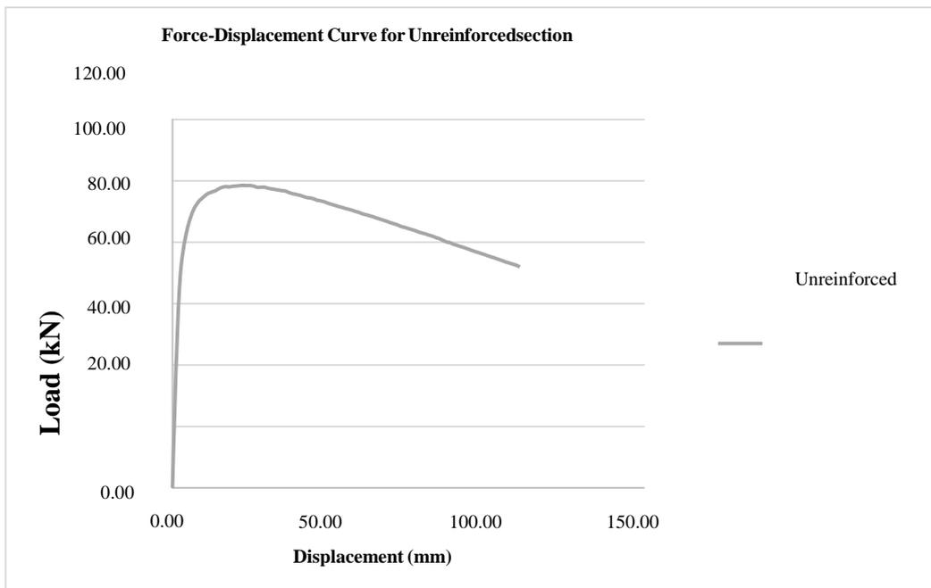
Figure 4.4 Force-Displacement Curves for Unreinforced Section
