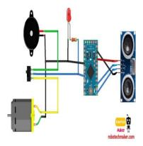
Working: This proposed system consists the equipment like Arduino Nano, ultrasonic sensor, bread board, buzzers for detecting the obstacles and letting the user know about the obstacle, Red LEDs, Switches, Jumper cable, power bank, Male and female header pins, some elastic and stickers to make the device wearable as a band for wearing for the users. The wiring of the device is done in a following manner. The Ground of LED, buzzer are
