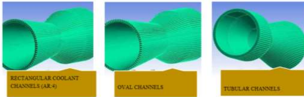
Fig 2.1 Patterns of coolant channels
