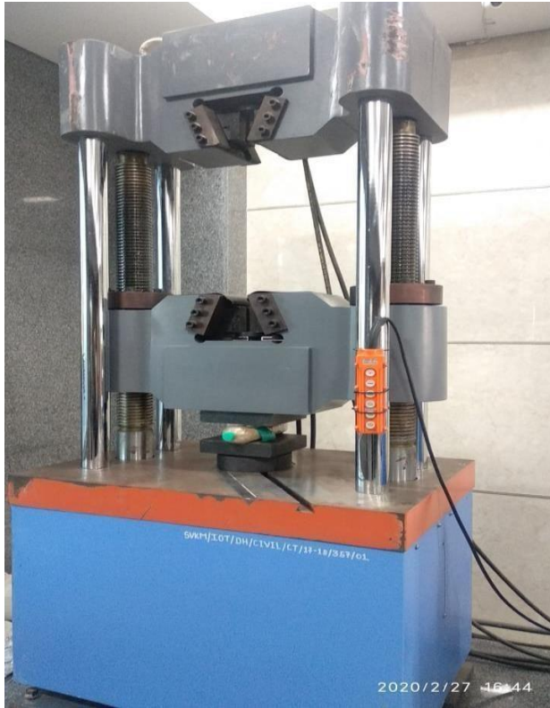
Fig 4- Crushing test on a plastic bottle fly ash
