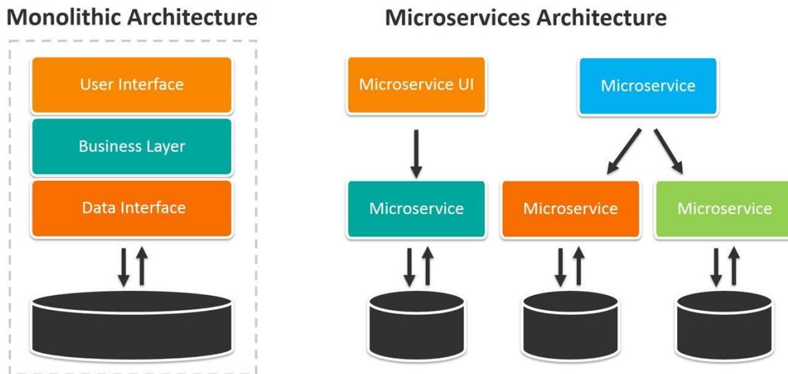
Figure 4.1: Monolithic Architecture Vs Microservice Architecture
