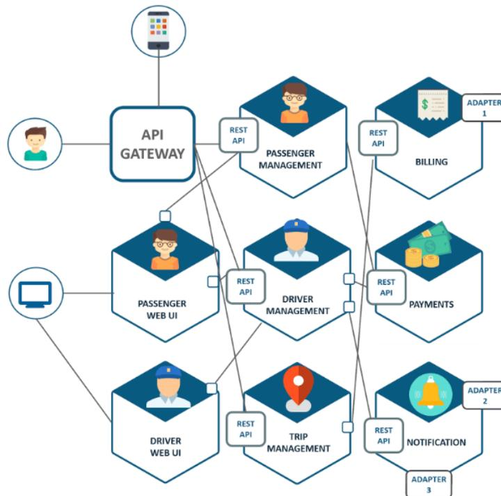
Figure 6.5: Uber's Microservices Architecture
