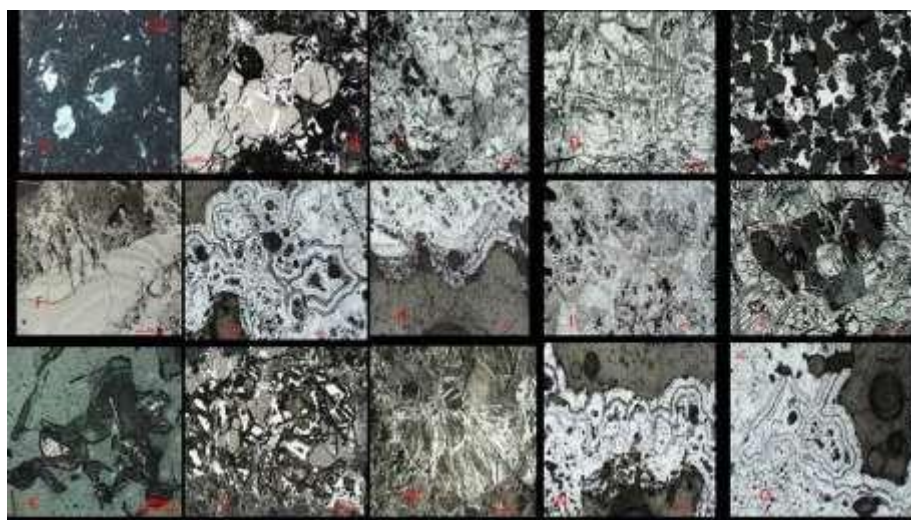
Figure 5: A) Cryptomelane replacing plagioclase B) Extremely fine grained cryptomelane replacing country rock along cracks as veins C) Psilomelane showing characteristic growth texture. D) romanchite (mammillary structure) cross cut by the psilomelane veins E) relict silicate structure concentration of pyrolusite F) Psilomelane colloform banding G) Birnessite alteration product of Mn oxide precursors, hydrothermal H) Birnessite (lighter grey fibres) alteration product of Mn oxide precursors, indication of deep sea hydrothermal alteration I) Polianite brownish and greyish pleochroism associated with Goethite (dark grey) J) Garnet (spessartine) replaced by Rhodonite K) garnet and magnetite in quartzite L) Replacement texture of cryptomelane M) Symplectite intergrowth between braunite and hausmannite N-O) banded colloform texture of pyrolusite & Psilomelane
