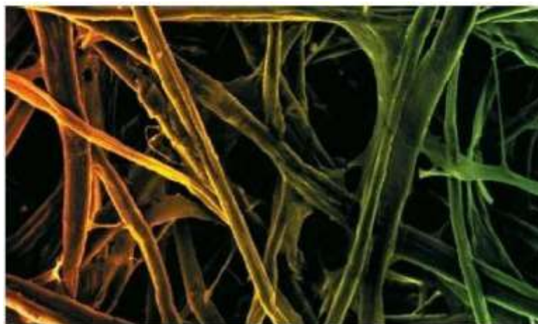
Fig.2.5 Appearance of pine apple fiber under scanning electron microscope
