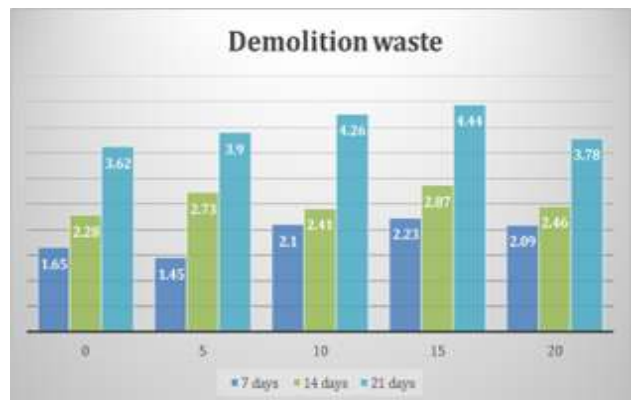
Split tensile strength of concrete by Demolition waste with cement kiln dust
