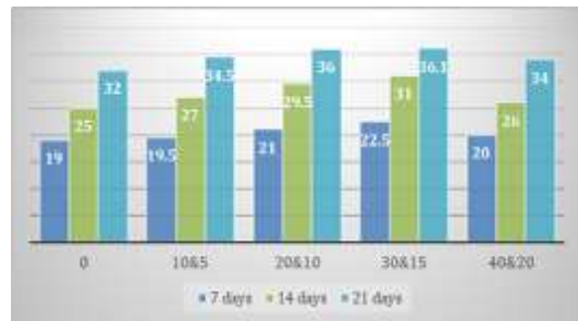
Compressive strength of concrete by partial replacing sand and cement
