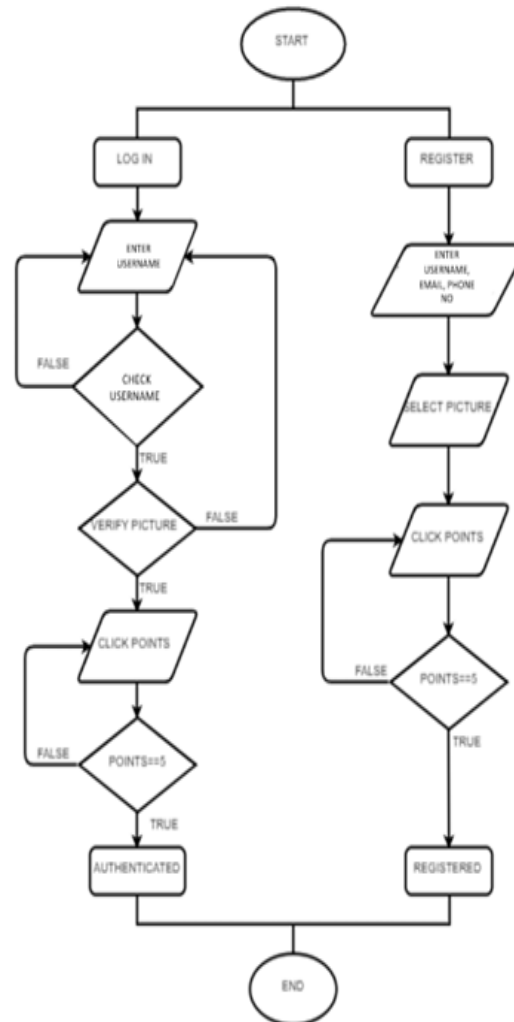
Flowchart for Graphical Password Authentication Using PassPoints Method
