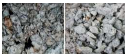
Fig. 2-(b) Before and after coating of plastic waste to aggregates
