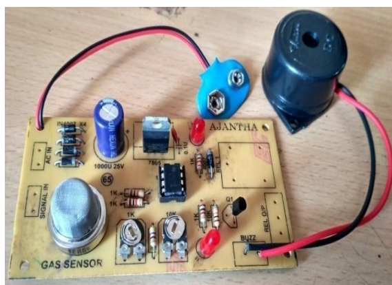
LED and Buzzer. As a result, the LED will glow and the buzzer starts to produce alarm sound.
