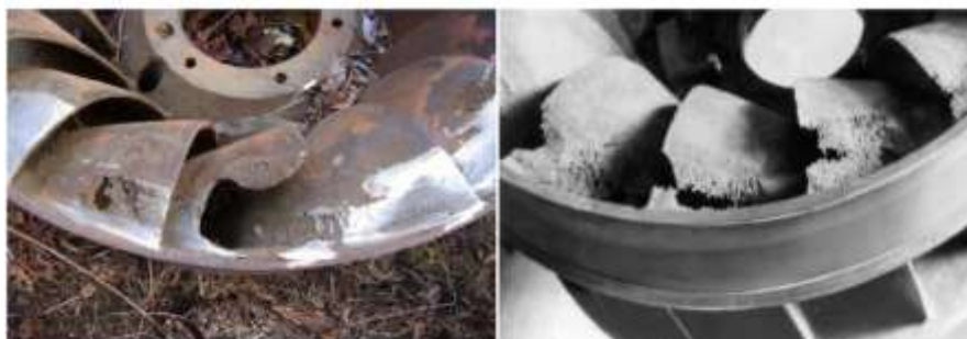
Fig:Turbine cavitations due to vibrations
