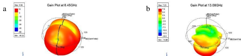
Fig 6. Gain plot of Circular patch Antenna without unit cell (a) Gain at 6.45GH is5.66dB, (b) Gain at 13.08GHz is 7.23dB.
