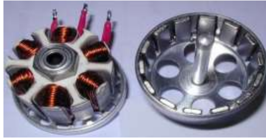
Figure 3: Brushless type Direct Current motor (stator and outer rotor)
