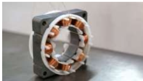
Figure 2: BLDC motor stator
