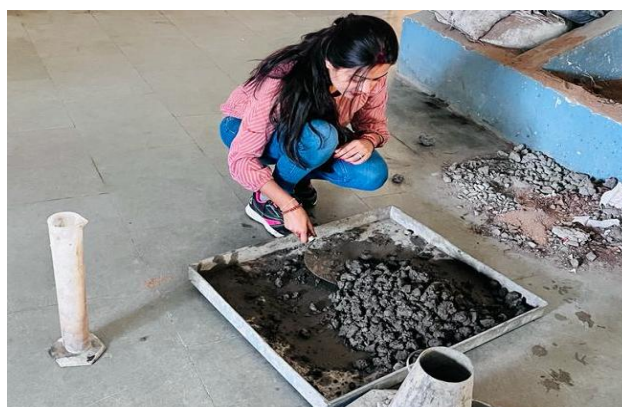
Figure 1: Casting specimen for test on hardened concrete.
