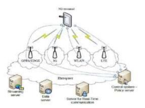
The system comprising of a main user terminal and then a number of independent and autonomous radio access technologies. Each of the radio technologies is considered as the IP link for the outside internet world. The IP technology is designed exclusively to ensure sufficient control data for appropriate routing of IP packets related to a certain application connections i.e. sessions between client applications and servers somewhere on the Internet.
