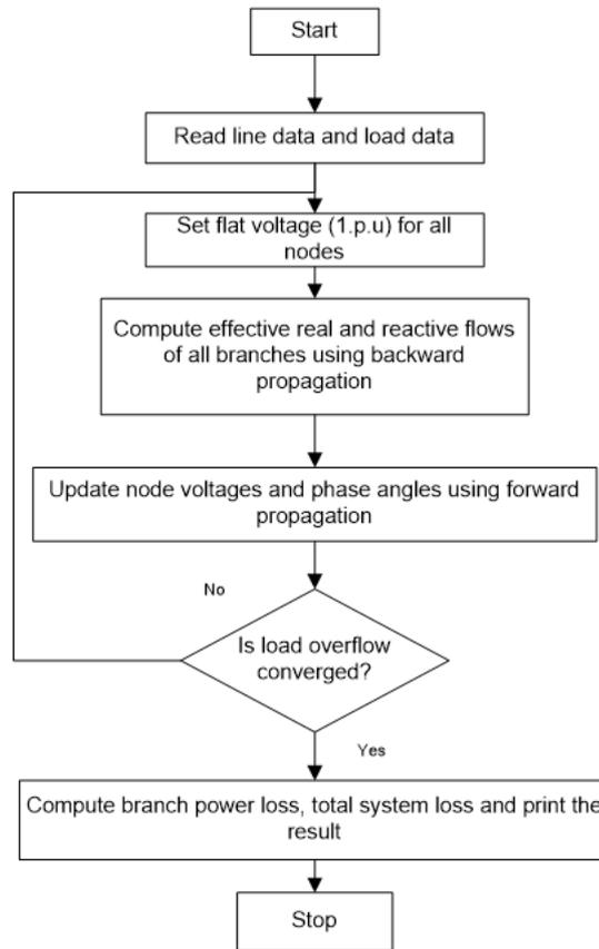
Fig 3.1: Flow Chart of Backward/Forward Sweep Method
