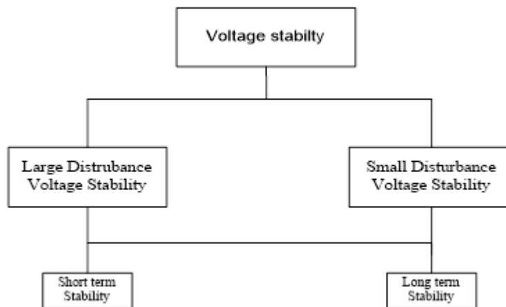
Fig 2.1: Classification of voltage stability
