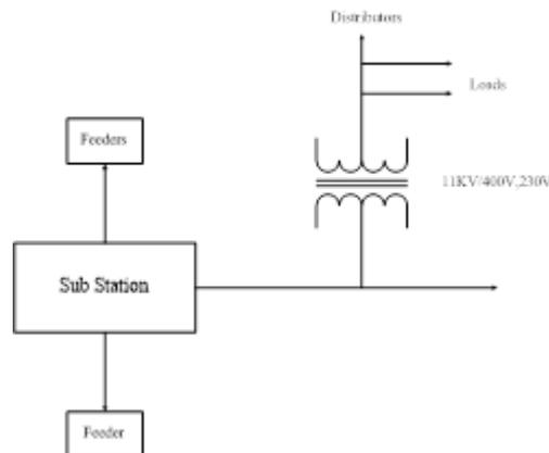
Fig 3.1: Radial distribution system
