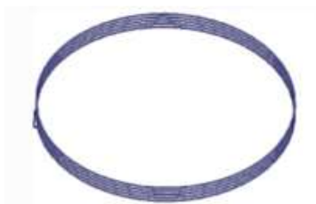
Fig. 8. Spiral coil design[1]
