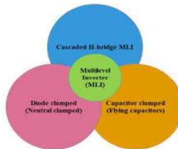
Figure-2 Topologies of multilevel inverter
