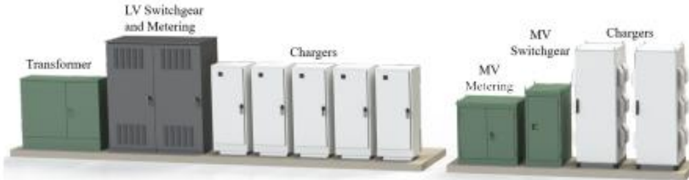
Fig. 5: Comparison of the state-of-the-art dc fast charger station to the SST-based solution. Both stations at rated at 675Kw
