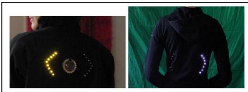
Fig. 7. Examples of jackets with turn signals powered by Lilypad Arduino sewn onto them
