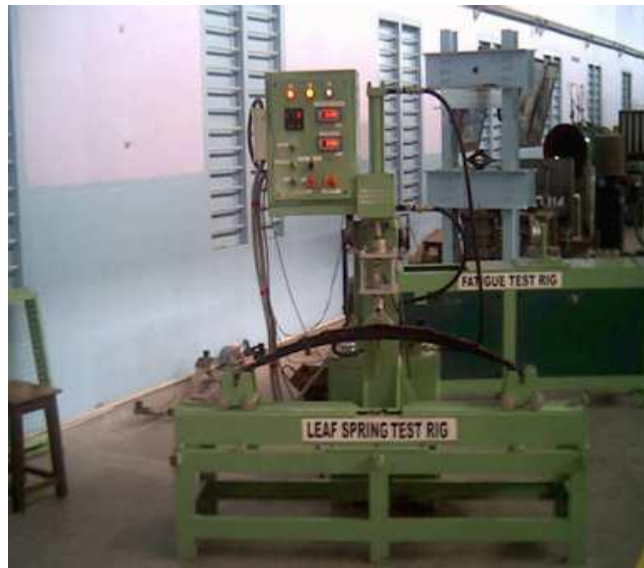
Fig. 5 Electro-hydraulic leaf spring test rig. [10]
