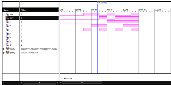
Fig 7: Simulation result for Reversible full adder.
