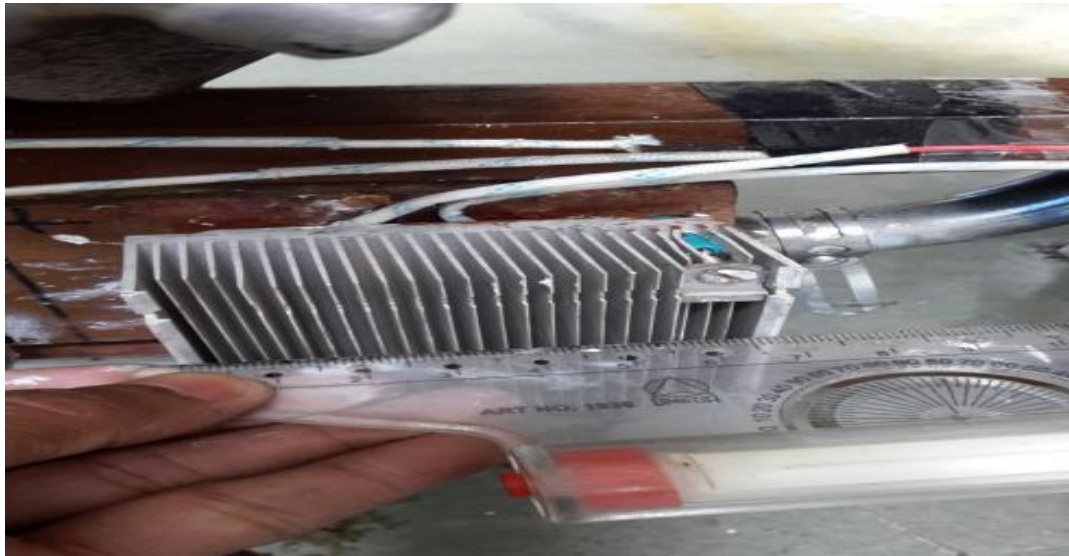
4.2 Aluminum heat sink fabricated for the present study
