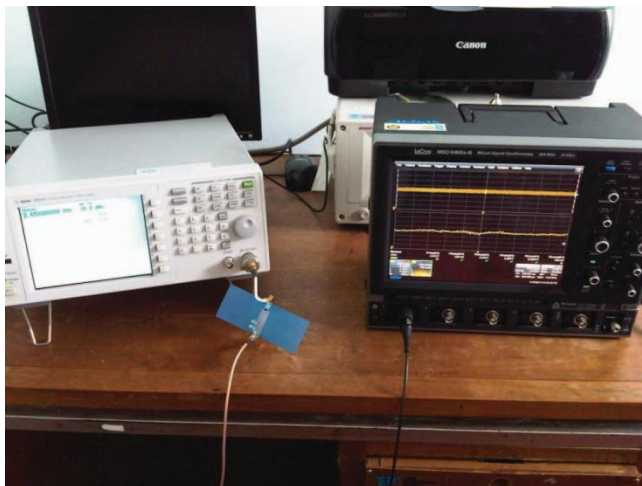
Fig. 7. Complete rectifier measurement setup.
