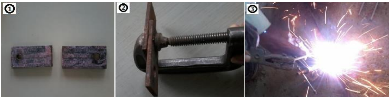
Fig.4.4 Procedure for overlap length specimen preparation
