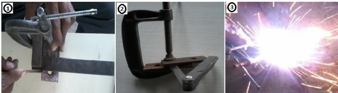
Fig.4.6 Procedure for gap size specimen preparation
