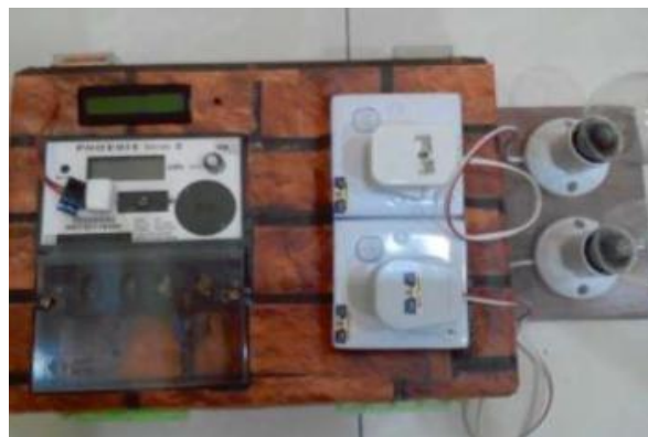
Figure 2: Energy meter with loads of 2 lamps
