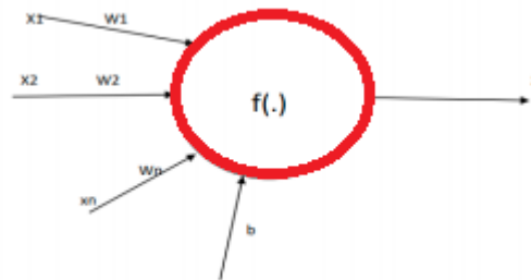
Figure 1: A Simple Artificial Neuron with Inputs and Output predicting layer as z.
