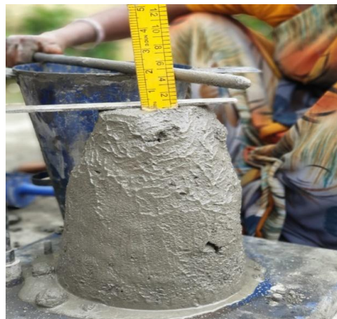
Figure 3.1: Slump cone test
