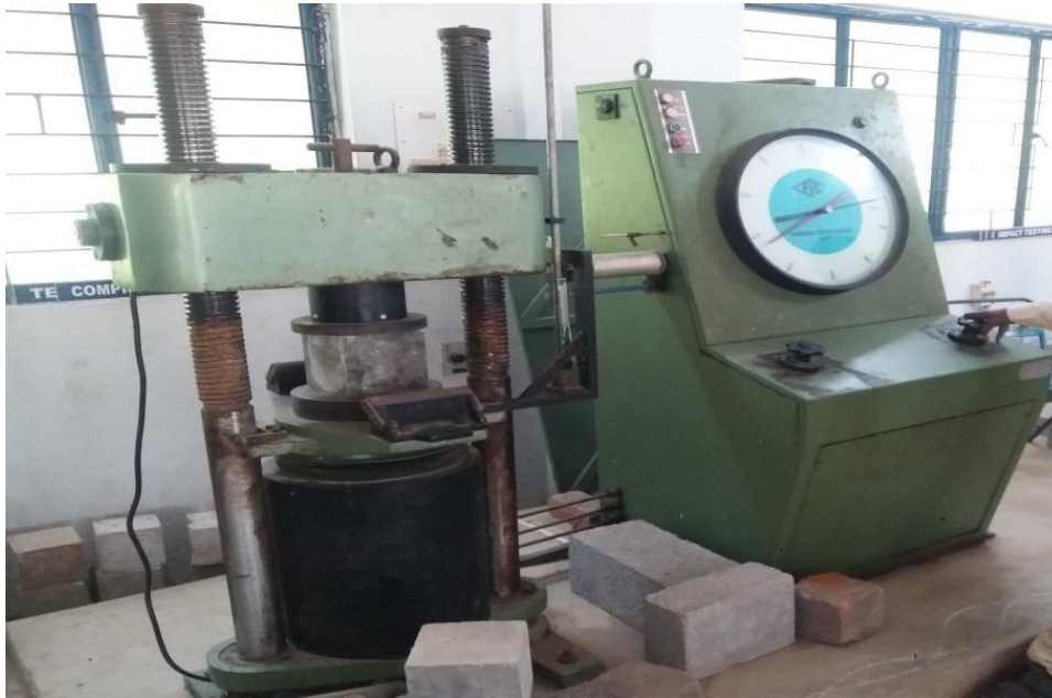
Figure 3.2: Experimental set up to find the compressive strength of concrete
