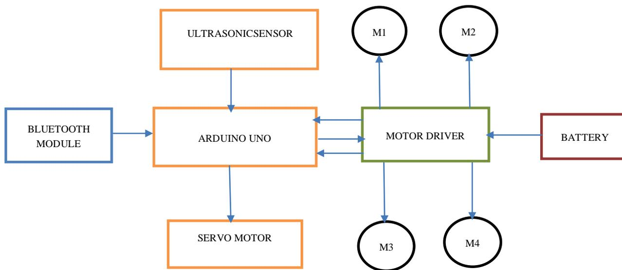
Fig. 1–voice controlled robot vehicle block diagram
