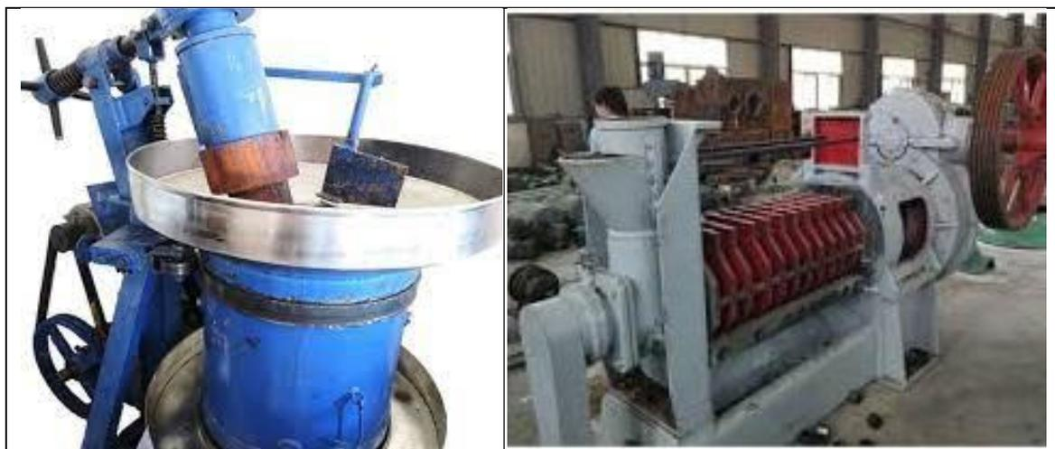
**Fig 3: Oil Extraction by (Ghani) and Electric Extractor**
