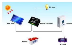
Fig.1 Solar cell PV system
