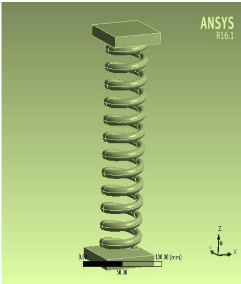
Fig. 3 3D model of compression helical spring
