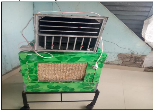
Fig. 18 Experimental Working of the Duct rotating air cooler
