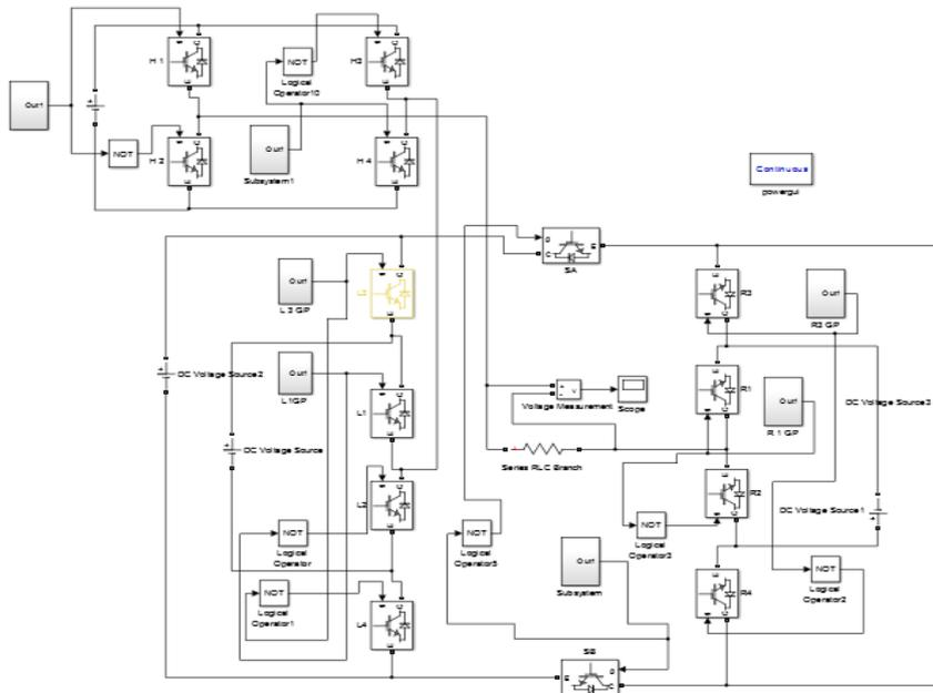
Fig.2. Simulation Model of the proposed cascaded MLI
