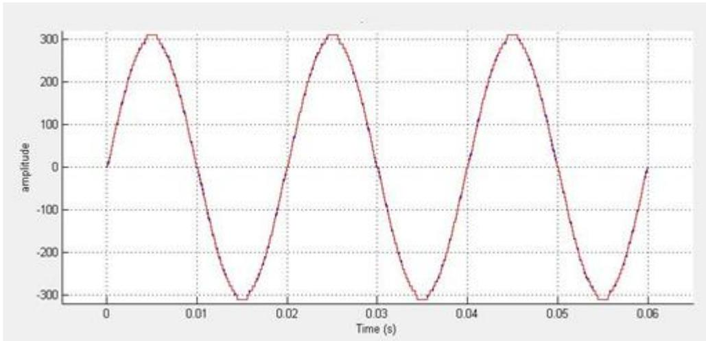
**Fig. 14 Sixty-three level output Voltage of overall cascaded MLI**
