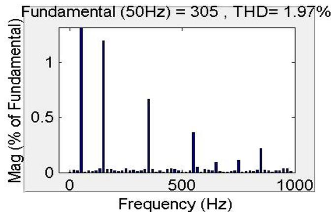
Fig. 15 FFT analysis of overall cascaded MLI
