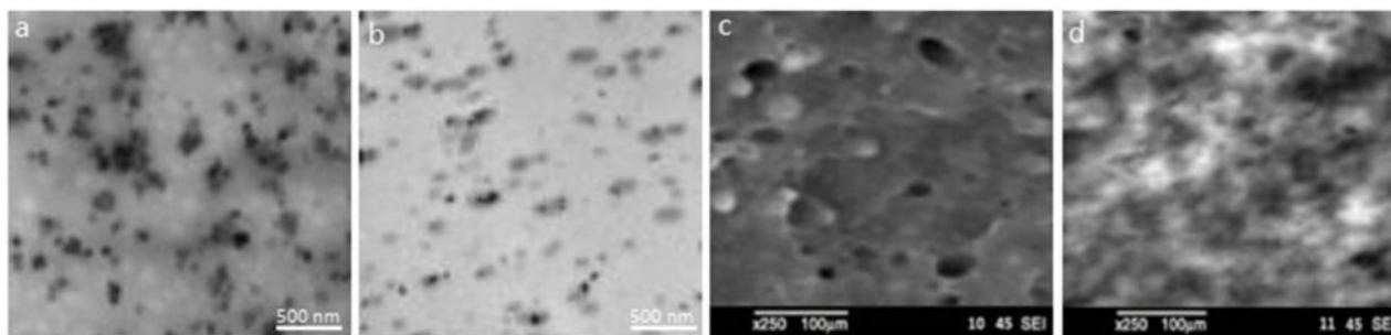
**Fig. 2-** TEM images of (a) TPE/3UnTiO<sub>2</sub> and (b) TPE/3CnTiO<sub>2</sub> nanocomposites and SEM images of (c) TPE/3UnTiO<sub>2</sub> and (d) TPE/3CnTiO<sub>2</sub> nanocomposites.
