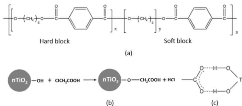
**Scheme 1- (a) Basic structure of thermoplastic polyester elastomer (TPE); (b) surface modification of  $\text{TiO}_2$  with chloroacetic acid (c) binding mode of carboxylate with titania surface: hydrogen bonding.**
