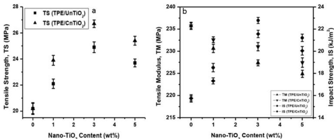
Fig. 1- (a) Tensile strength and (b) tensile modulus and impact strength of TPE/nTiO<sub>2</sub> nanocomposite.
