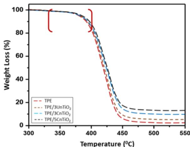
Fig. 3- TGA curves of pure TPE and TPE/nTiO<sub>2</sub> nanocomposites.
