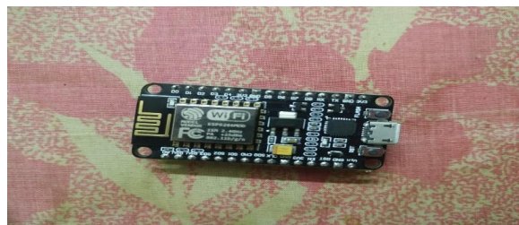
Fig. 1 - ESP8266 NODE MCU WIFI SOC
