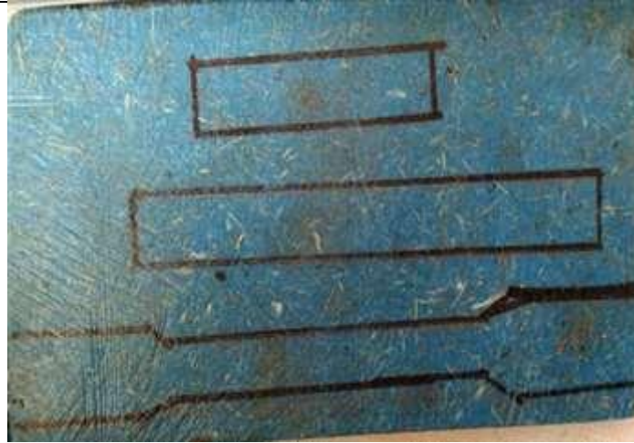
Fig 8 .Speciman marking for Tensile, Flexural and impact test.
