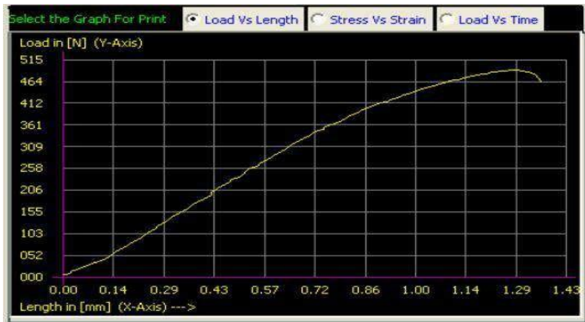
Figure 6: Bending Test Specimen 1
