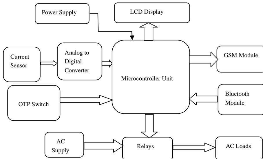
The system has a current sensor which will give load current value. Output of the CT is analog, so we have to connect a ADC in order to convert it in 8 bit Digital. This is done by using a ADC0808. Output of ADC can be fed to the microcontroller. Microcontroller will display the current value on a 16\*2 LCD. The controller will also compare it with the maximum allowable current value. If it is greater than that then the relay will get tripped automatically.
